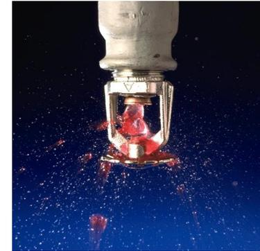
2- Heat expands the liquid, the air is compressed and the glass shatters
