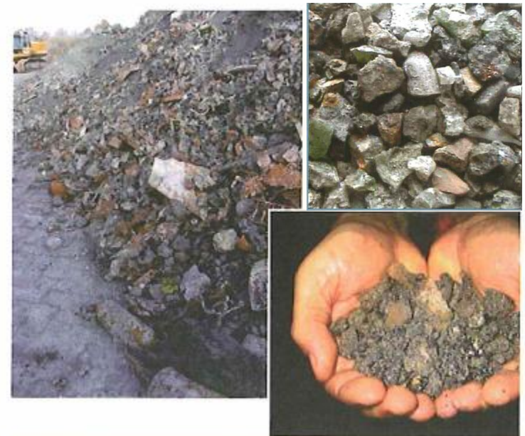
Figure 2: Examples of raw incinerator bottom ash (left) and the ash after the ferrous metal has been removed (right)
