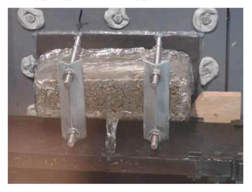
Michelmersh facing brick under test. 3.5 l/hr seepage at 1m head of water.
