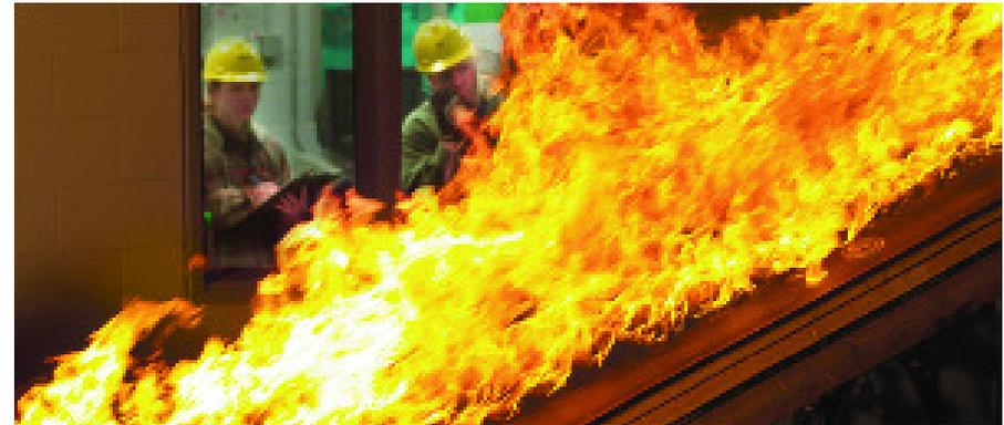
These are large scale tests using a re-entrant corner (as per BRE testing).
