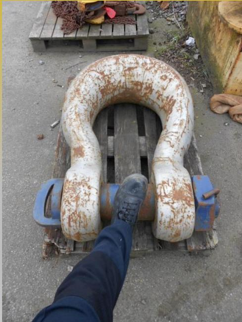
This Shackle has a Lifting Capacity of 1400 tonnes and takes 4 men just to put the pin in!
