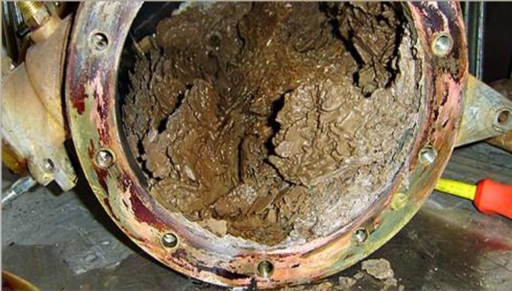
This is scale inside a coffee boiler that built up over a period of 9 months
