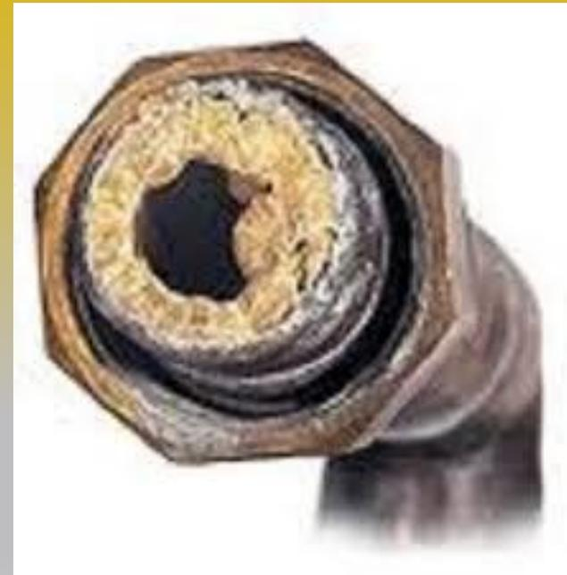
A Badly Limescale damaged valve restricting flow of water into boiler
